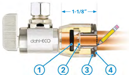
EPDM O-RING | STEEL TEETH | LOCKING CLIP | RELEASE SLEEVE
