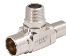
616SS-13-62 1/2 Fem. Solder x 3/8 MIP, Loose Key w/Screwdriver Operation
